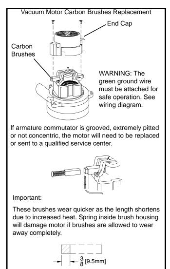
Periodically check the length of the carbon brushes. Replace both carbon brushes when either is less than 3/8" (9.5mm) long.
